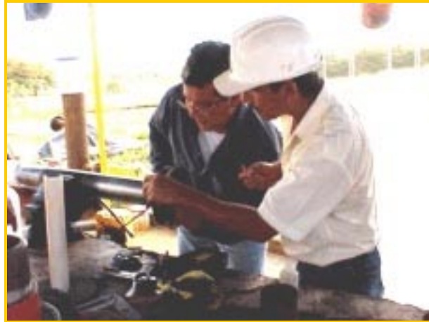
Figure No.5 – Measuring the Remaining Wall Thickness in Defect “B”
