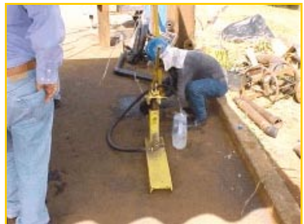
Figure No. 14 – Testing Baker Pump
